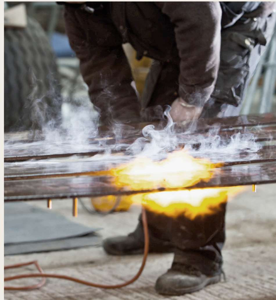
Warming the Corten to speed the patination process.
