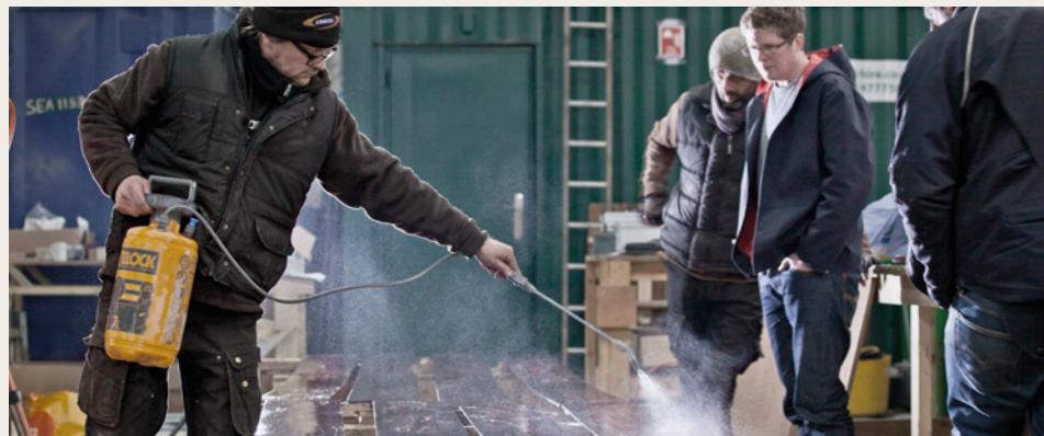
Above: Removing the stencil and counters prior to burnishing the copper.
